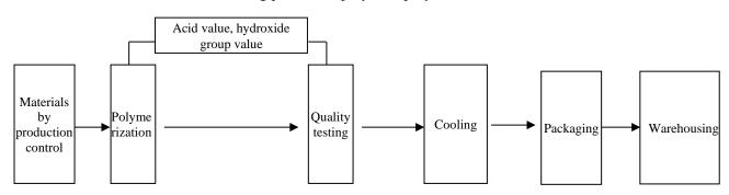
(3) Manufacturing process of polyurethane granules (hot melt adhesive and shoe adhesive)
